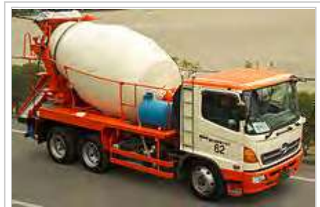
This Kayaba Rocket concrete mixer delivers concrete in Japan.
