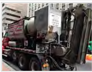
Metered concrete truck
