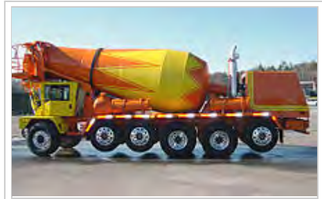
Terex Advance front discharge truck with three lift axles including one tag axle
