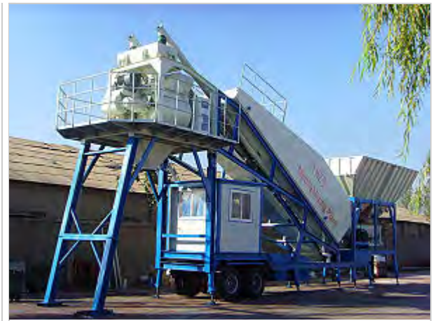
Mobile concrete plant is a kind of special construction equipment, which is developed for construction and emergency repair of airport runways, roads, bridges and other concrete work.
