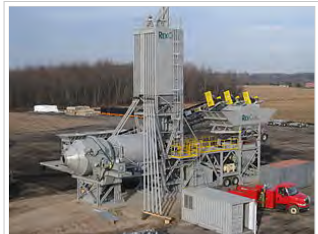
RexCon Model S portable concrete paving plant with dual mixers can produce up to 55 loads of concrete per hour, or around 550 cubic yards per hour, from a single lane of traffic.
