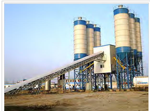
A typical non-North American design of concrete plant. Longer conveyors and screw-fed cementitious materials slow down production significantly.
