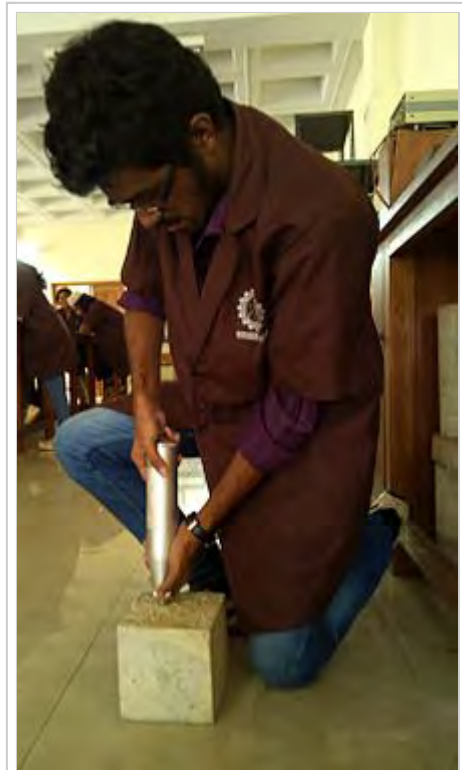
Testing the compressive strength of a concrete cube using Schmidt hammer
