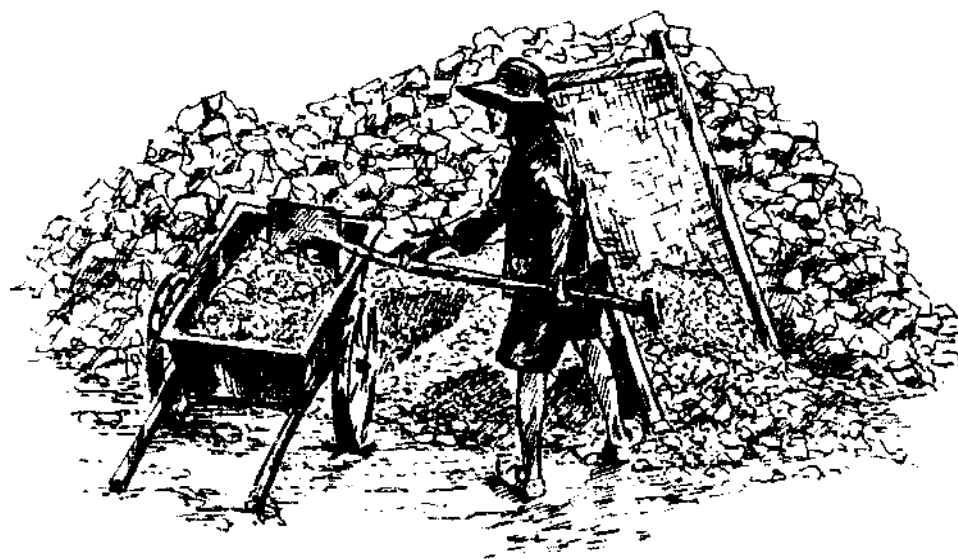
Using a coarse sieve for low grade dry hydrate.
