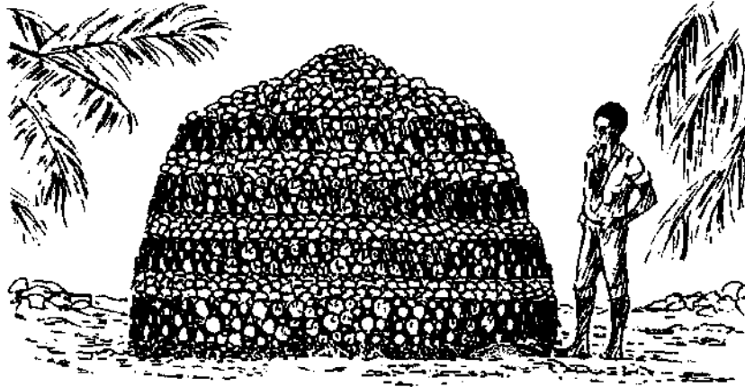
An uncovered heap with alternative layers of wood and limestone.
