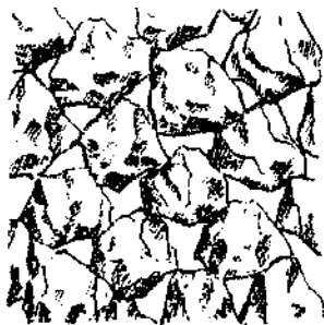
Good voids between equal-sized lumps.
