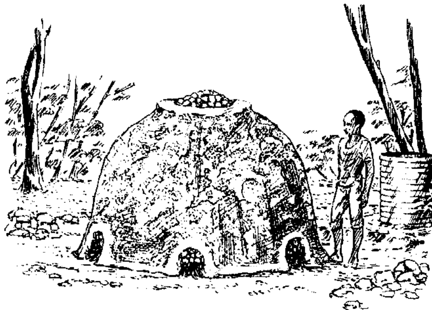
A heap covered with clay daub.
