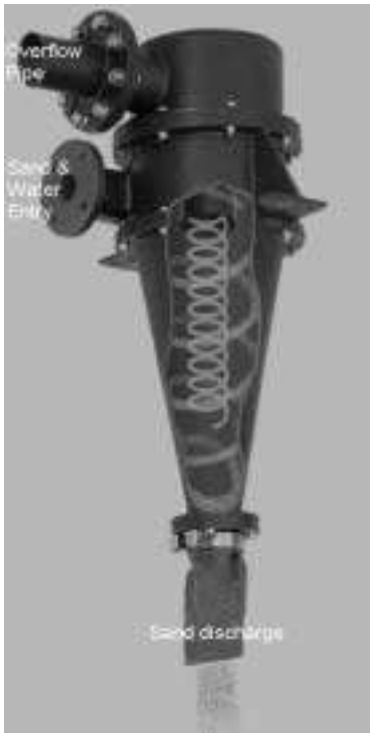
Figure 1.2: A Hydro-cyclone
