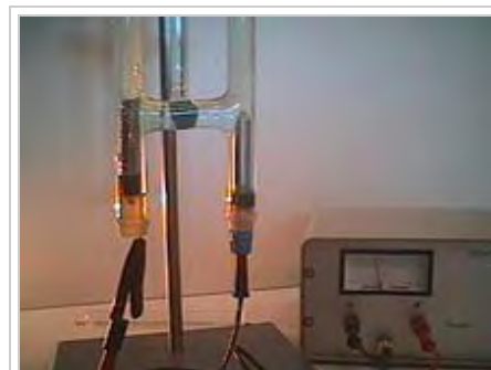
Hoffman voltameter connected to a direct current power supply
