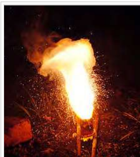
An exothermic thermite reaction using iron(III) oxide. The sparks flying outwards are globules of molten iron trailing smoke in their wake.
