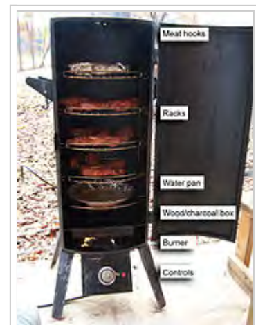
A diagram of a propane smoker used to prepare smoked foods
