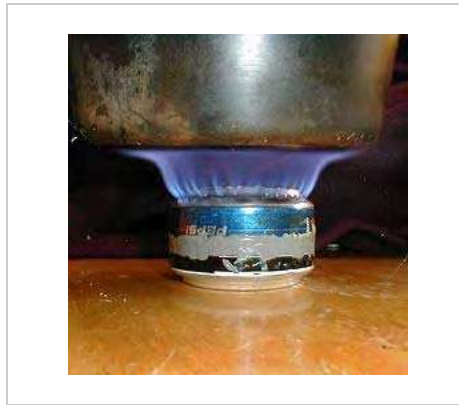
A beverage-can stove; the pot stand is omitted for clarity
