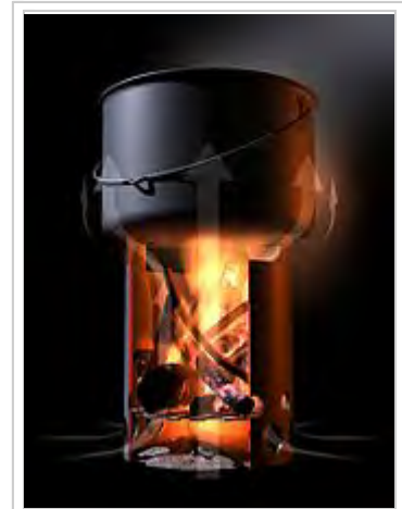
Heat convection in a hobo stove (schematic)
