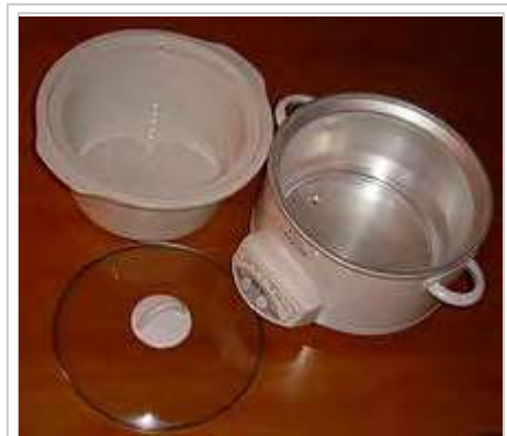
A newer slow cooker. This one has a removable ceramic "crock" (upper left), glass lid (lower left), and heater –housing (right) with push button controls, instead of the original single knob.
