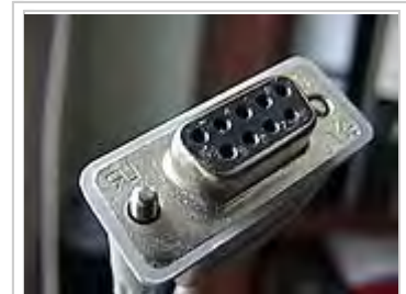
A fire control system's RS-232 data connection which an emergency communication system may interface with
