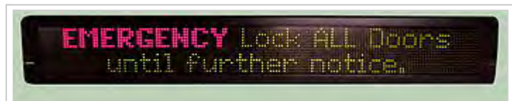
LED sign, in a wall-mounted orientation, depicting an emergency and the resulting action that should be taken to mitigate the emergency
