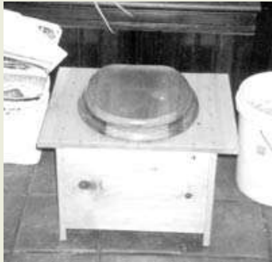
LIFT-OFF SAWDUST TOILET IN RURAL HOME
