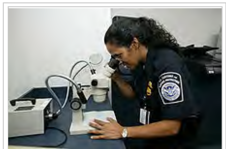
CBP Office of Field Operations agent checking the authenticity of a travel document at an international airport using a stereo microscope
