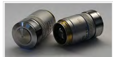
Two Leica oil immersion microscope objective lenses: 100 \times (left) and 40 \times (right)
