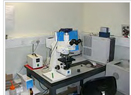
A modern microscope with a mercury bulb for fluorescence microscopy. The microscope has a digital camera, and is attached to a computer.
