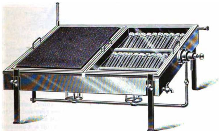
FIG. 41.—Hearson's apparatus for the coagulation of serum.
