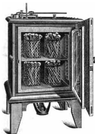
FIG. 49.—Hearson's "warm" incubator arranged to work with gas.
