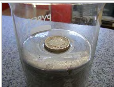
A pound coin (density \sim 7.6\text{ g/cm}^3 ) floats in mercury due to the combination of the buoyant force and surface tension.
