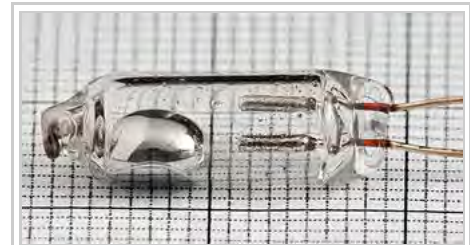
A Single-Pole, Single-Throw (SPST) mercury switch.
