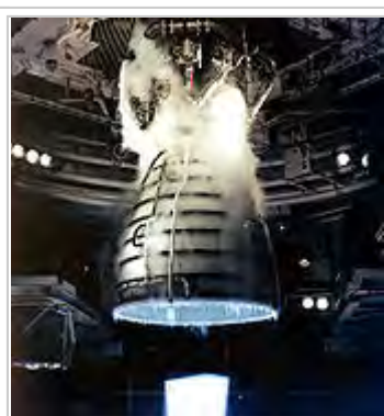
The Space Shuttle Main Engine burnt hydrogen with oxygen, producing a nearly invisible flame at full thrust.
