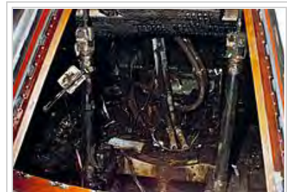
The interior of the Apollo 1 Command Module. Pure O 2 at higher than normal pressure and a spark led to a fire and the loss of the Apollo 1 crew.
