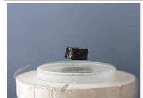
A typical event described by physics: a magnet levitating above a superconductor demonstrates the Meissner effect.
