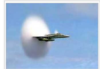
U.S. Navy F/A-18 approaching the sound barrier. The white halo is formed by condensed water droplets thought to result from a drop in air pressure around the aircraft (see Prandtl-Glauert Singularity). [9]
