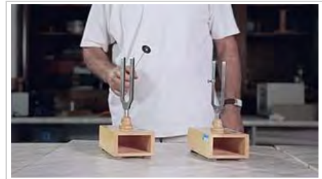
Experiment using two tuning forks oscillating at the same frequency. One of the forks is being hit with a rubberized mallet. Although the first tuning fork hasn't been hit, while the other fork is visibly excited due to the oscillation caused by the periodic change in the pressure and density of the air by hitting the other fork, creating an acoustic resonance between the forks. However, if we place a piece of metal on a prong, we see that the effect dampens, and the excitations become less and less pronounced as resonance isn't achieved as effectively. Performed by Prof. Oliver Zajkov at the Physics Institute at the Ss. Cyril and Methodius University of Skopje, Macedonia.
