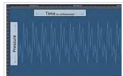
A 'pressure over time' graph of a 20 ms recording of a clarinet tone demonstrates the two fundamental elements of sound: Pressure and Time.
