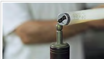
A Tesla coil producing high-frequency current that is harmless to humans, but lights a fluorescent lamp when brought near it (experiment performed by Prof. Oliver Zajkov at the Physics Institute at the Ss. Cyril and Methodius University of Skopje, Macedonia)
