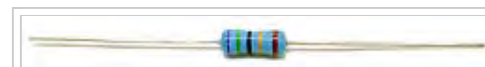
A 6.5 MΩ resistor, as identified by its electronic color code (blue–green–black–yellow). An ohmmeter could be used to verify this value.
