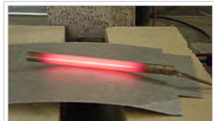
Running current through a material with high resistance creates heat, in a phenomenon called Joule heating. In this picture, a cartridge heater, warmed by Joule heating, is glowing red hot.
