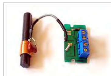
LC circuit ( left ) consisting of ferrite coil and capacitor used as a tuned circuit in the receiver for a radio clock.
