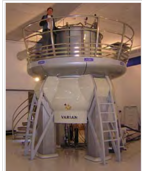
NMR Magnet at HWB-NMR, Birmingham, UK. In its strong 21.2-tesla field, the proton resonance is at 900 MHz.
