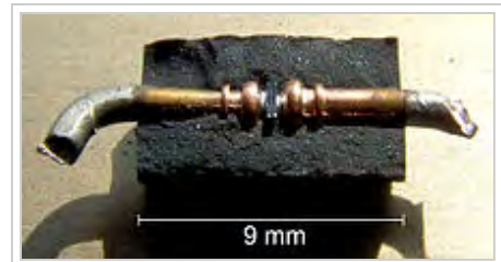
1N5822 Schottky diode with cut-open packaging. The semiconductor in the center makes a Schottky barrier against one metal electrode (providing rectifying action) and an ohmic contact with the other electrode.
