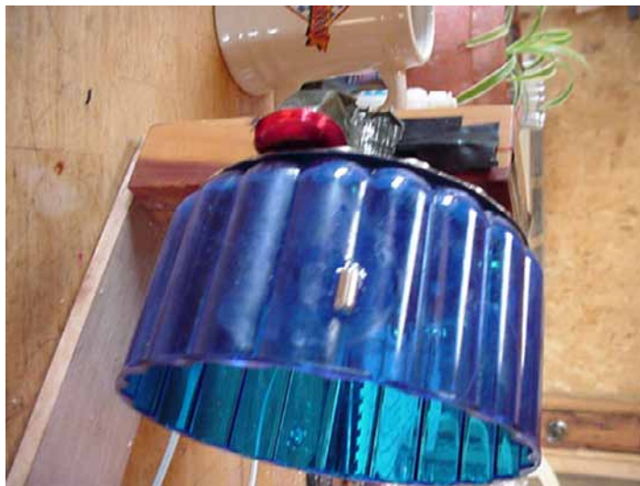
magnet trigger glued to outside radius of wheel
