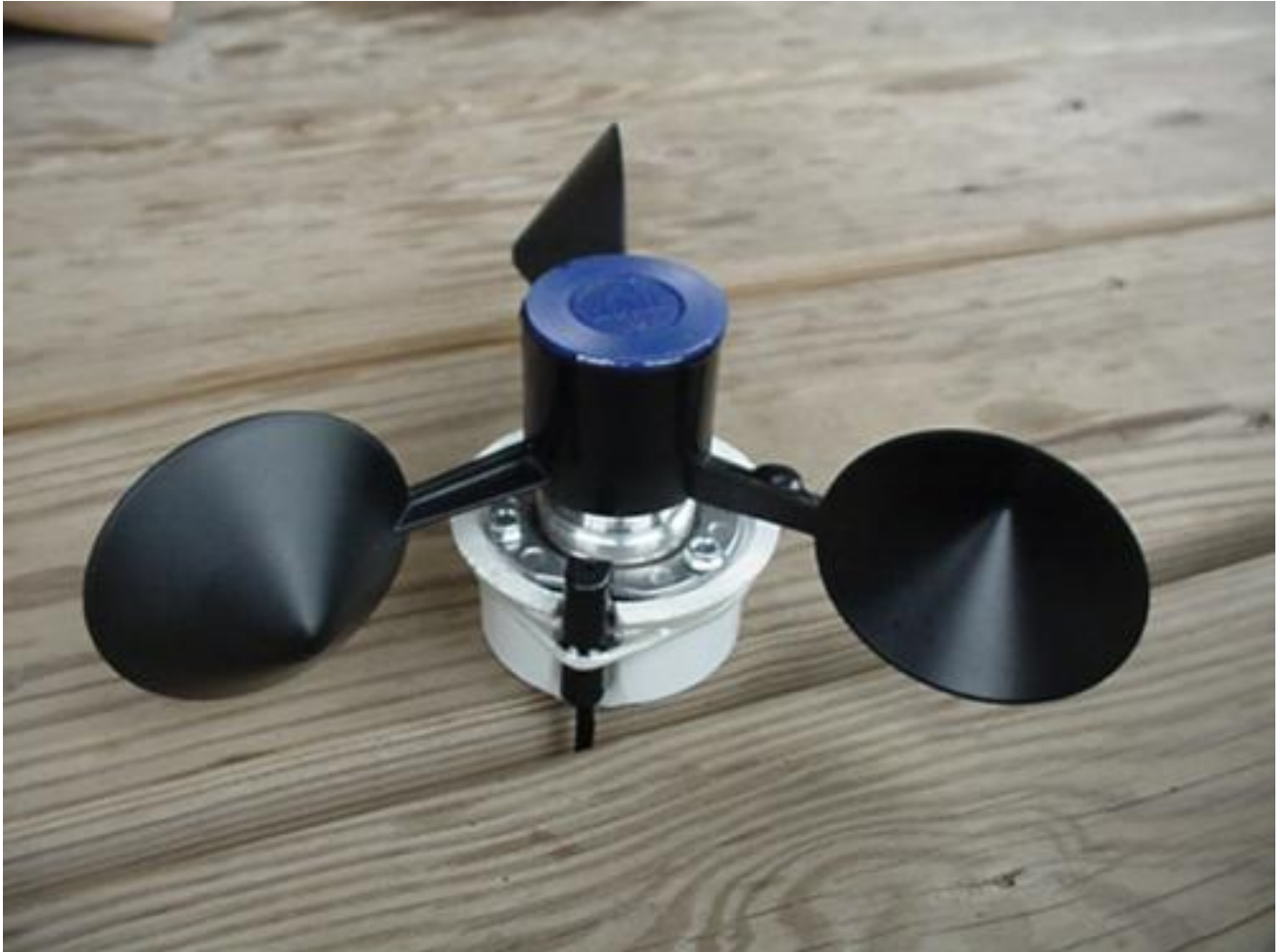
The completed anemometer cup and sensor assembly.
