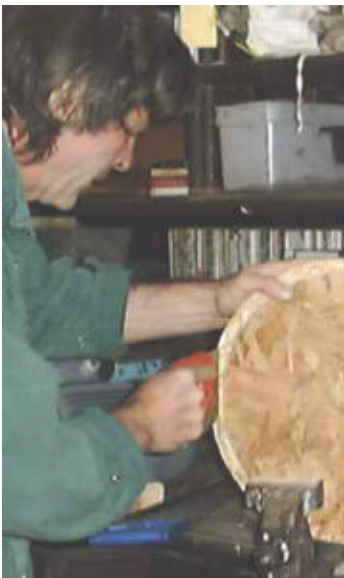
Sawing flat faces on the inner mould
