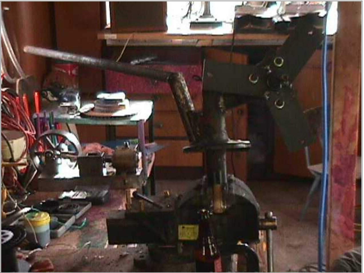
Pictured above the main chassis of the wind turbine is pretty much together. You can see now how the stator bracket bolts on. The tail boom is 5' long.
