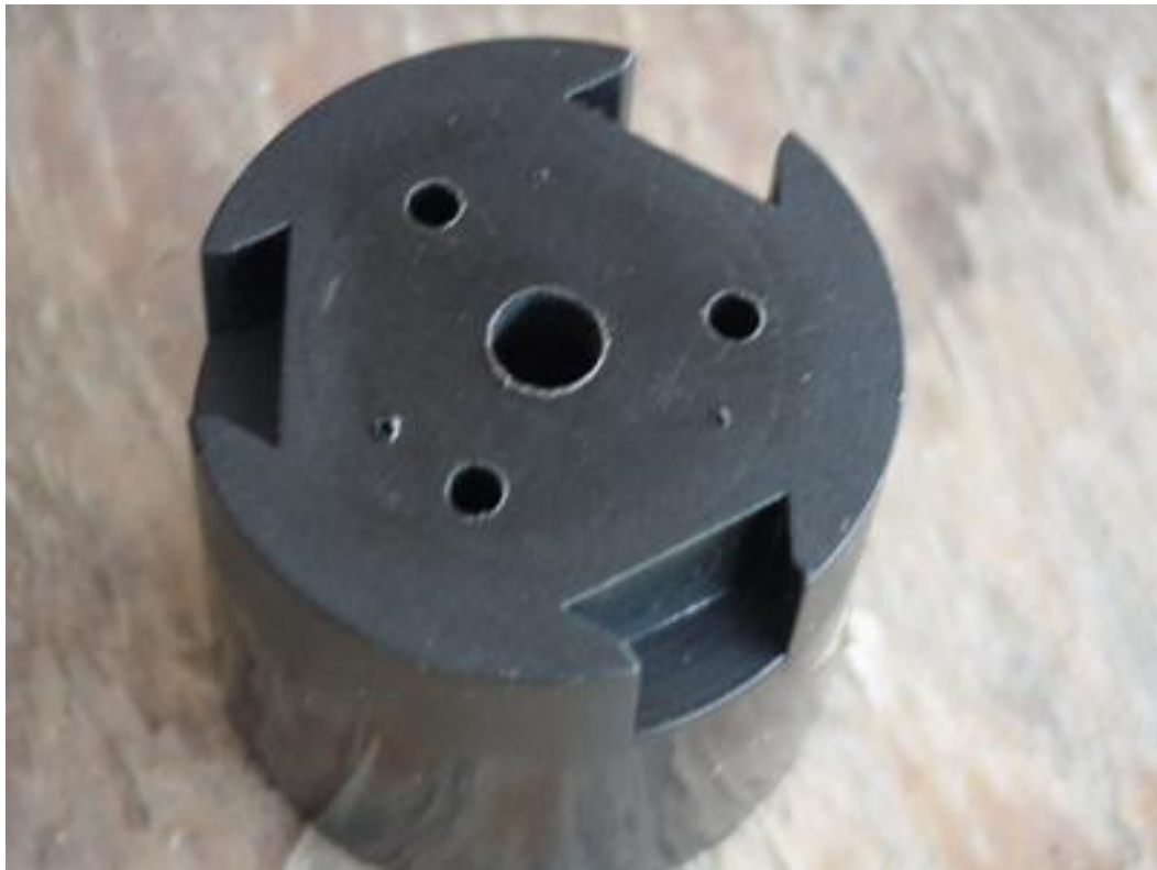
Completed anemometer hub assembly
