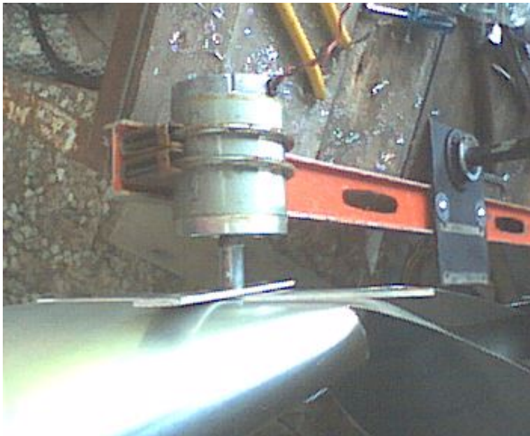
Tape Drive Motor mounting and pivot detail. Yes that is an aluminum 4 foot level.
