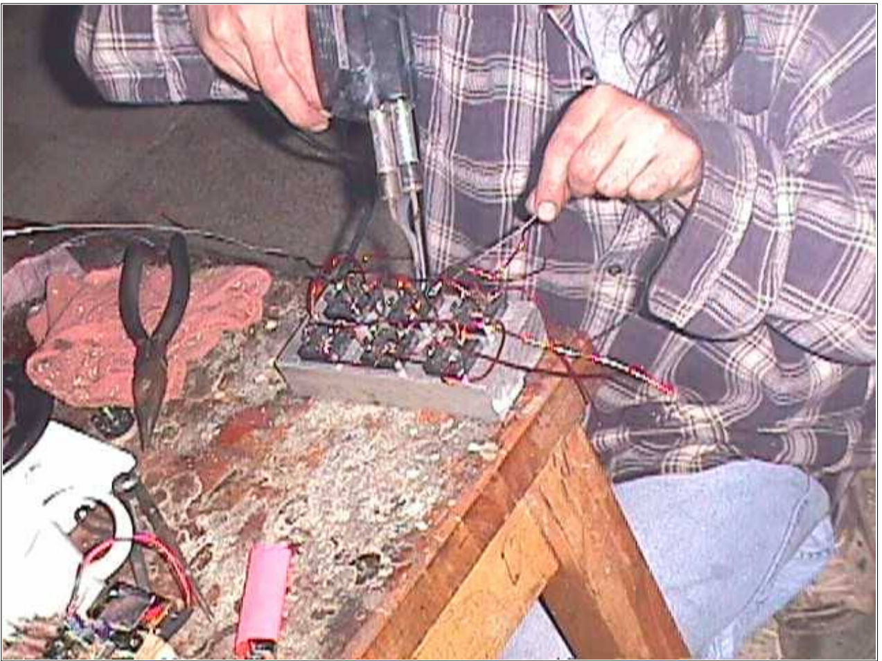
Here Dave is soldering up 6 bridge rectifiers we'll need in order to convert the 3 phase AC current into DC current useful for charging batteries.
