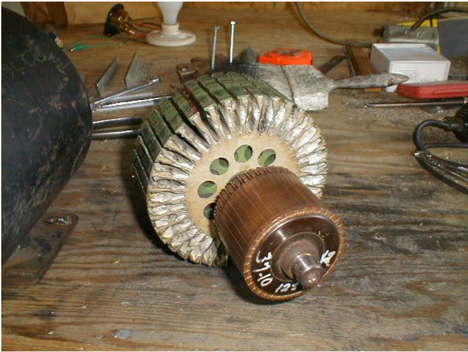
The stripped armature showing the large copper commutator and the armature slots ready for new coils.
