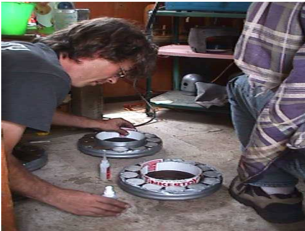
Pictured above I'm gluing up the inner part of the mold for the magnet rotors, made of a tinker toy can and playing cards. This holds the resin from leaking to the inside.
