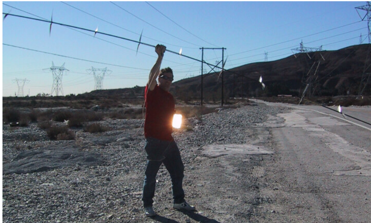
14 inch rotors lighting a 50 watt car headlight. More rotors = more power! So balanced it's comfortable to hold right in your hand - and very easy on the bearings!
