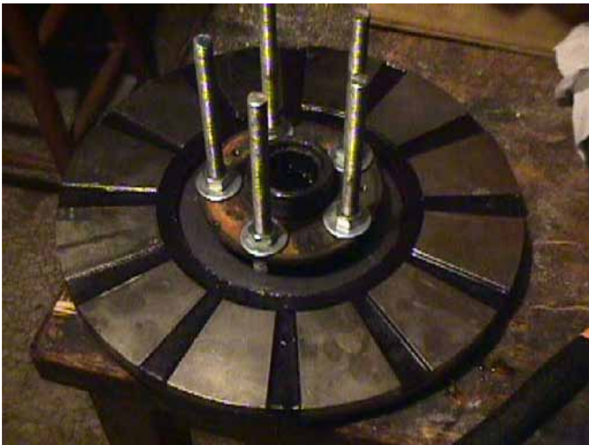
I cast the magnets in resin as shown above, and mounted the back rotor to the wheel hub.
