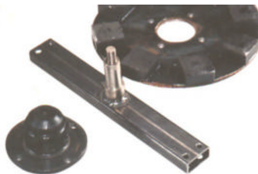
Spine, shaft, hub and magnet rotor
