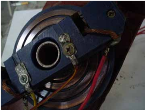
Here is showh assembled brush and sliding ring system.
