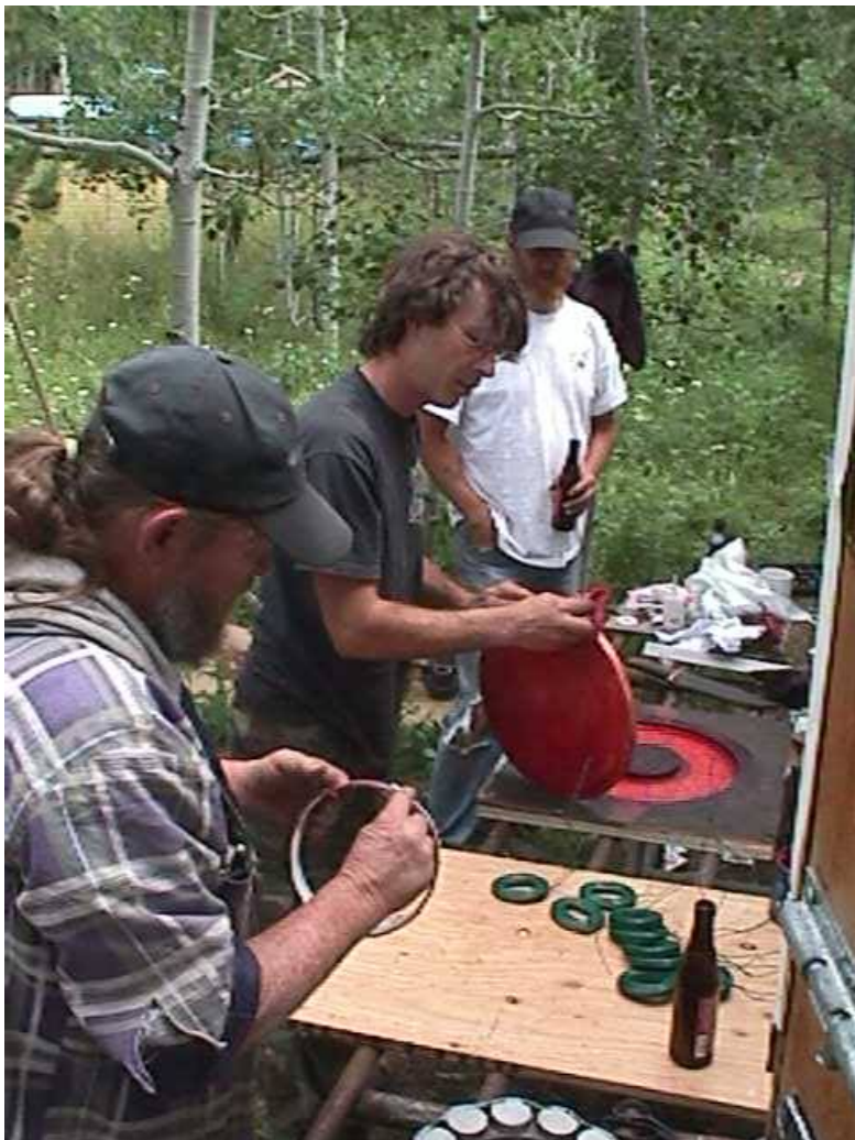
Pictured above I'm gluing up the inner part of the mold for the magnet rotors, made of a tinker toy can and playing cards. This holds the resin from leaking to the inside.
