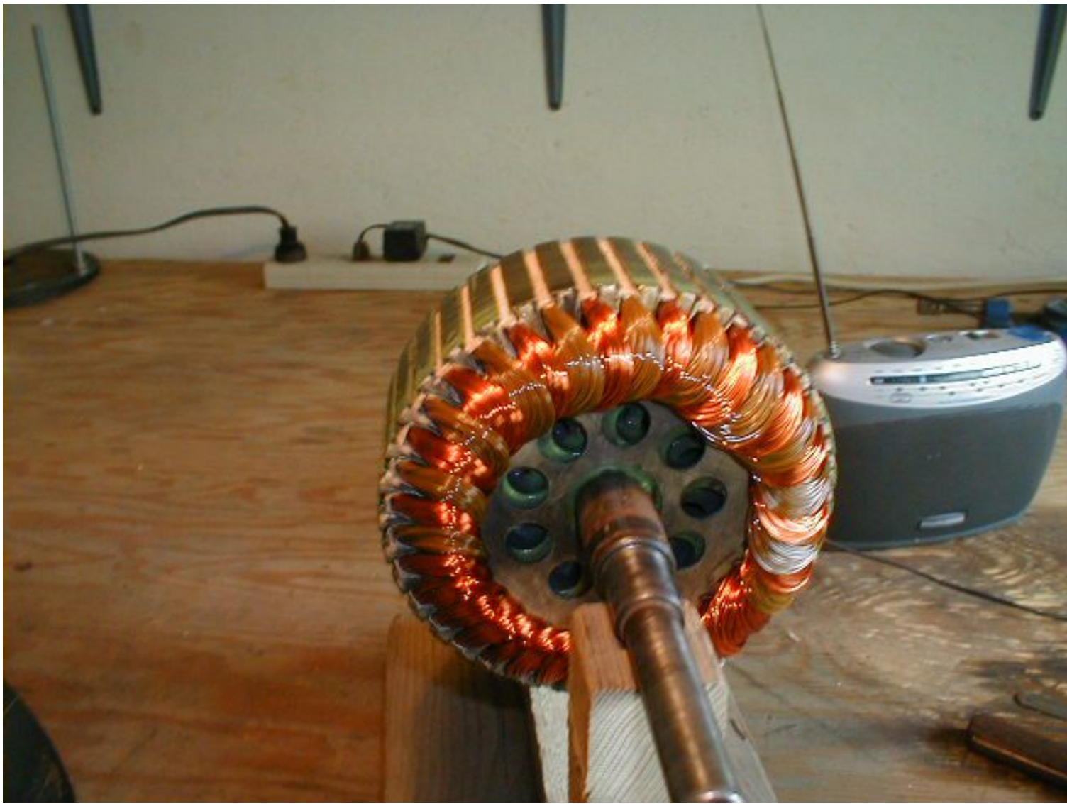
The semi finished back side of the armature. Note how the coils are bent over on each other to conserve space.
