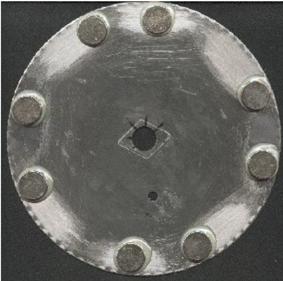
Dual Rotor, No Cog.. Nominal Output. Using saw blades for testing... Test Rig..
