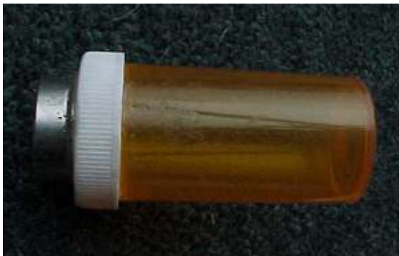
Float with magnet glued on top
