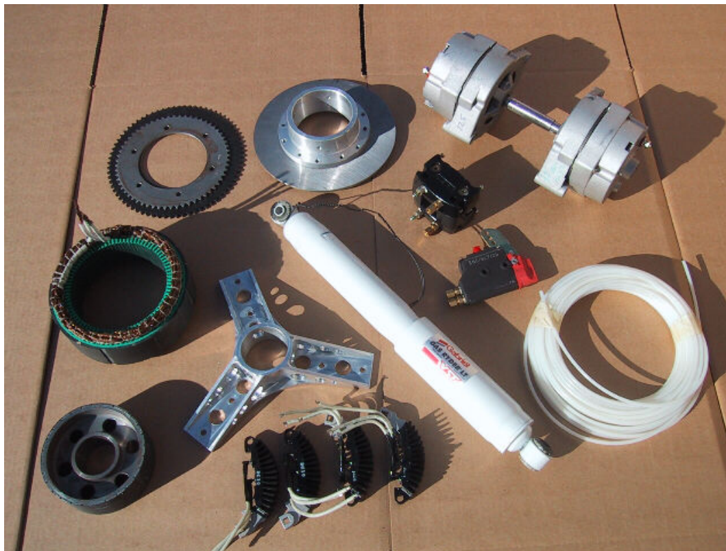
Parts is parts...hub, diodes, disk brake assembly, monoshock, alternators, and associated components
