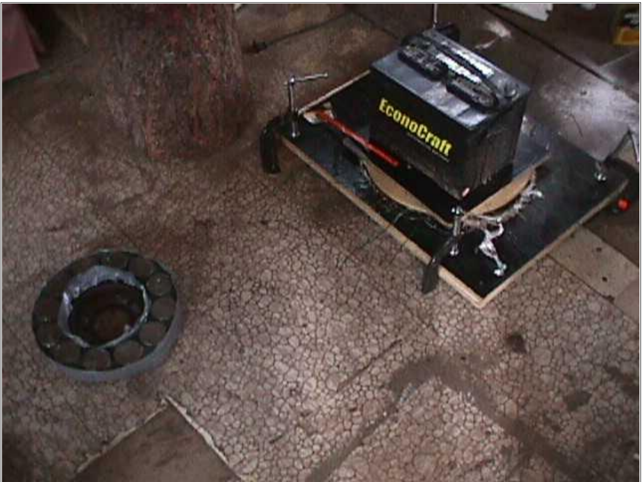
Here you can see the magnet rotor, and the stator mold while the resin sets up. The battery serves as a weight to hold the top of the mold down tightly.
