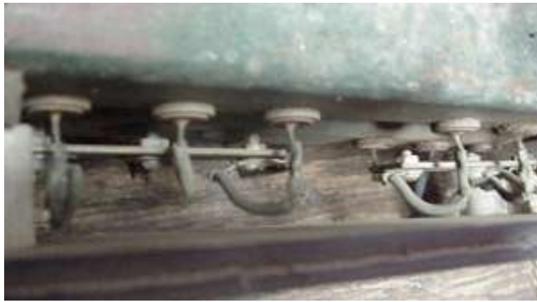
Close up of home built diode bridge
