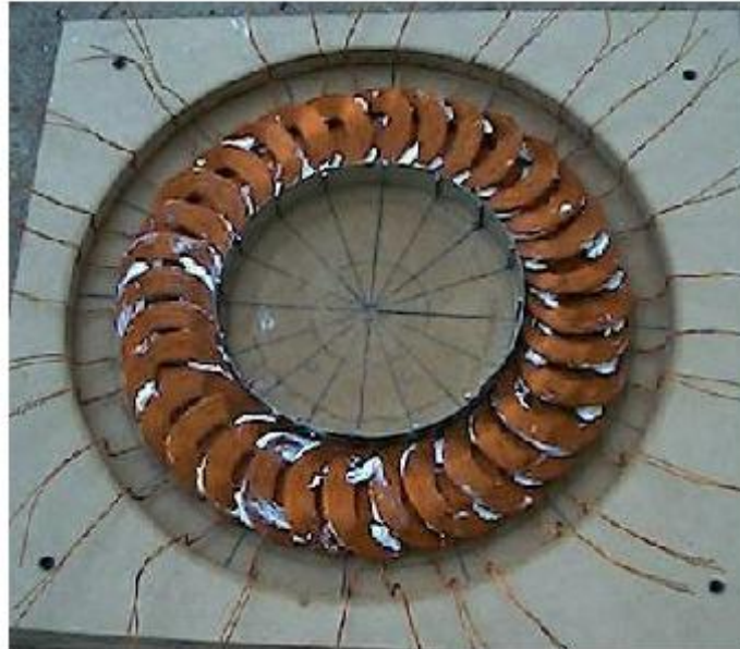
Step 2- Make some round center guide lines. make a sheet metal ring 1 inch in diameter, marked in red. the other two are center guide and outside coil diameter guide
