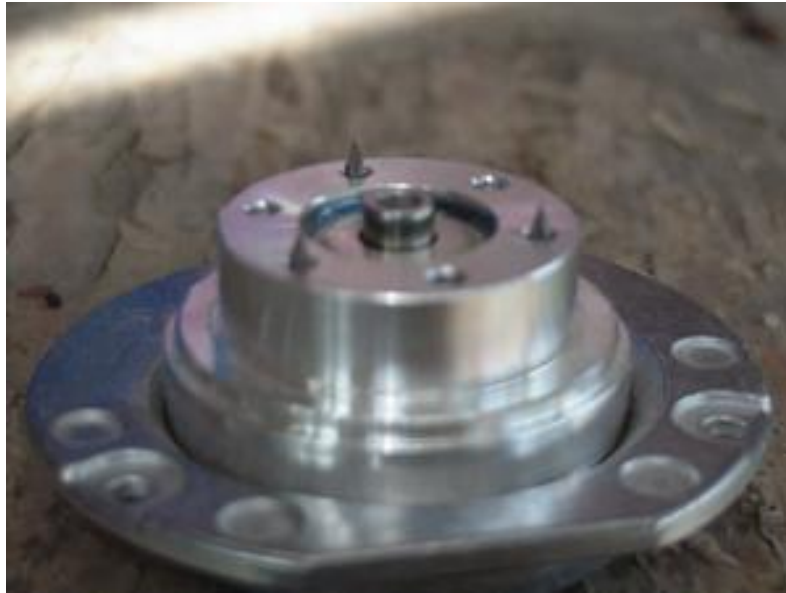
Nails in motor for marking hub holes.
