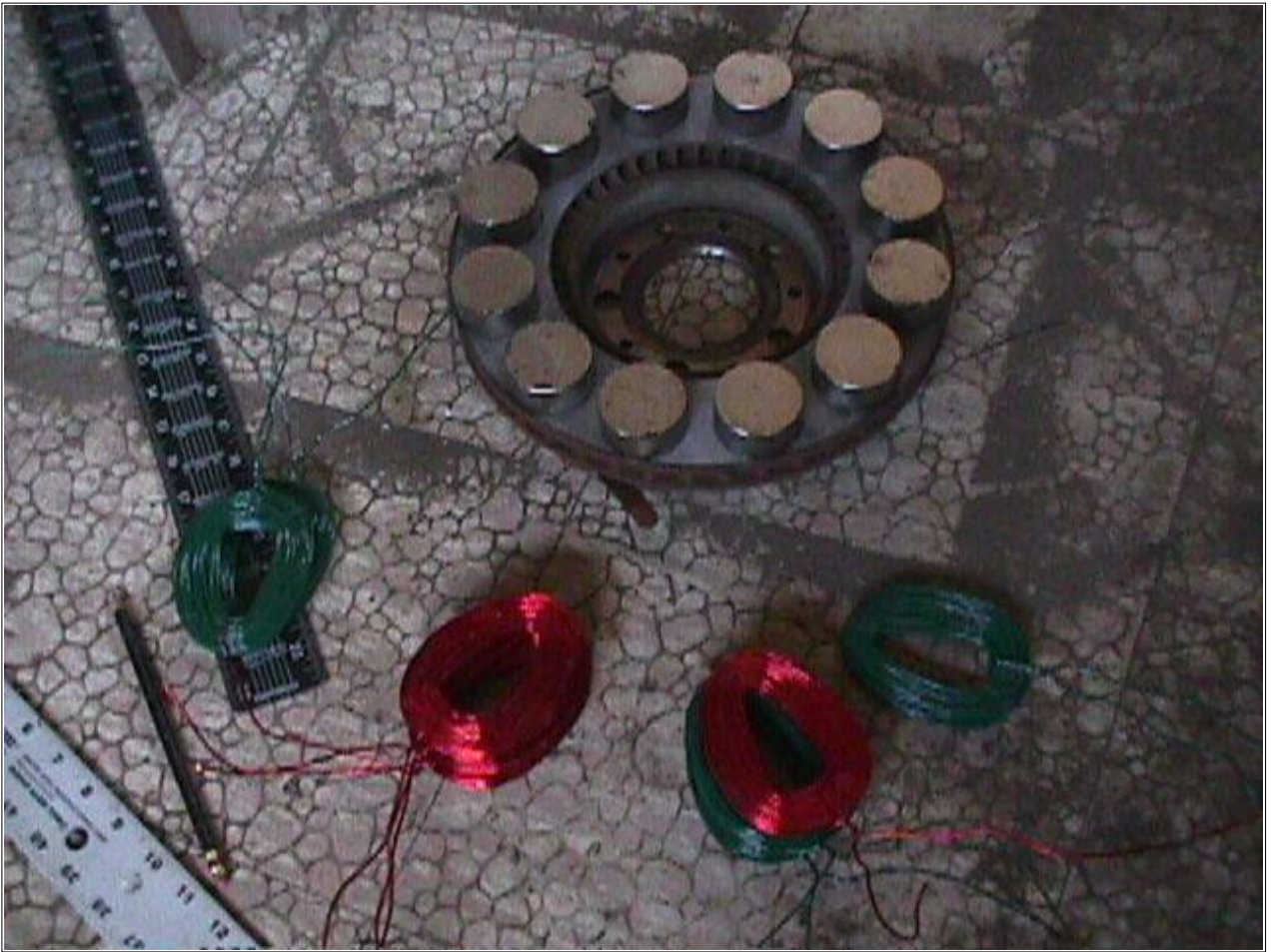
Pictured above are the coils, and the magnet rotor (the magnets are not glued down yet, actually I never did that till the very end and never got a picture of it finished).
