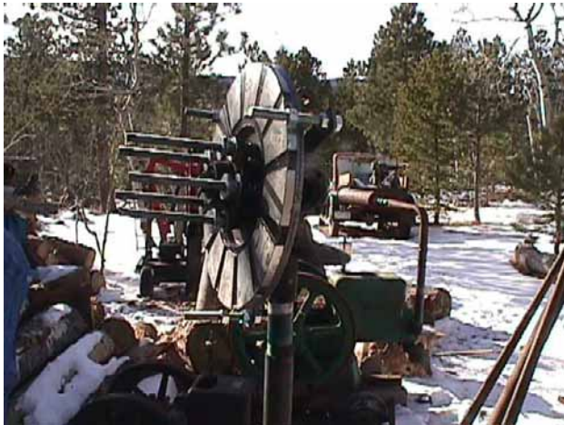
This picture shows how the back rotor of the alternator fits on the spindle.
