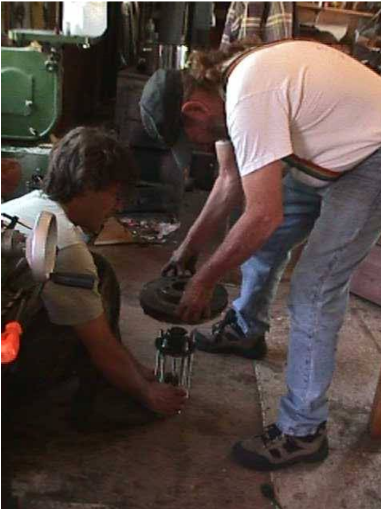
I'm holding down the wheel hub while Tom carefully lowers the magnet rotor
