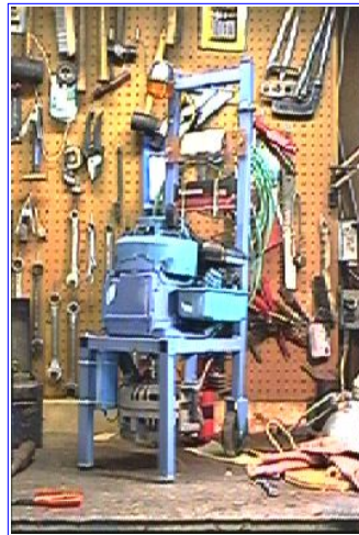
B&S/Chrysler Alternator 12 VDC @ 50 A
