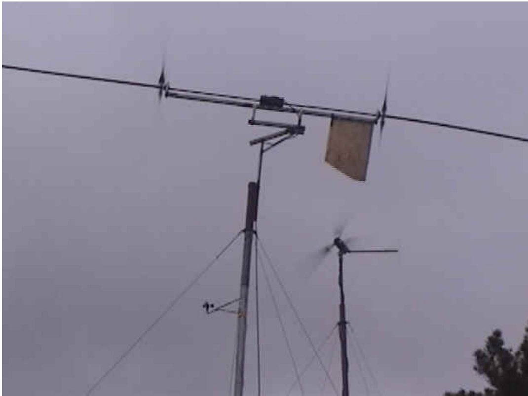
Selsam Turbine with four 4 foot diameter rotors furling to a horizontal configuration at about 30 mph, still producing full power. Downwind rotors are protected by the slipstream of the upwind rotor, limiting power production and thereby protecting from a runaway situation which would burn out the generator. This stops what would otherwise be a geometrically climbing power curve and begins to level it out above the rated wind speed. Conventional "1000 watt" turbine can be seen furling sideways in background, "cringing" at the force of this strong wind, and consequently producing very little electrical power when the wind speed is above the rated speed, where the best opportunity for producing power actually exists.
