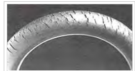
Ozone cracking in natural rubber tubing
