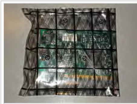
A network card inside an antistatic bag.
