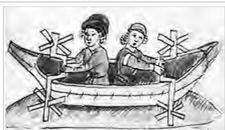
15th century paddle-wheel boat whose paddles are turned by single-throw crankshafts (Anonymous of the Hussite Wars)
