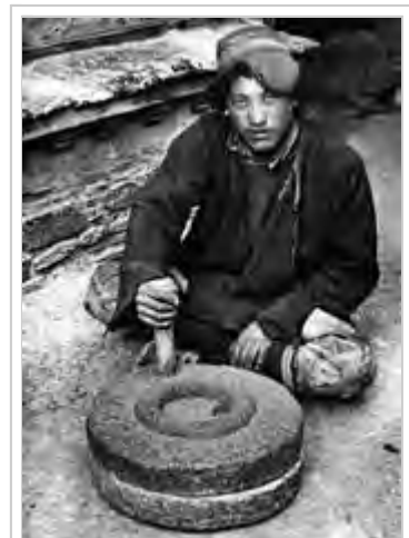
Tibetan operating a quern (1938). The upright handle of such rotary handmills, set at a distance from the centre of rotation, works as a crank. [3][4]
