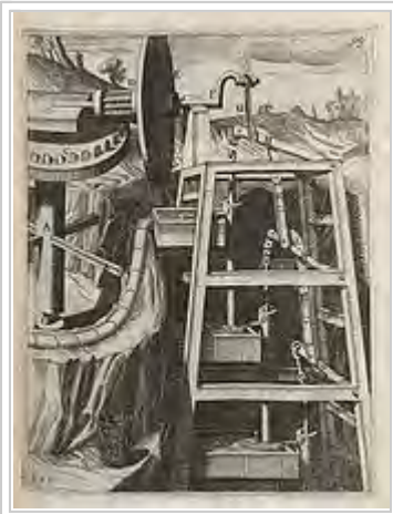
Water-raising pump powered by crank and connecting rod mechanism (Georg Andreas Böckler, 1661)
