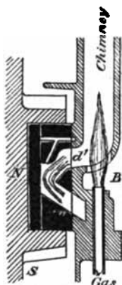
Fig. 40.—Ignition Flame and Slide Valve.
