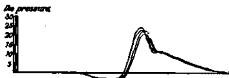
Fig. 7.—Hugon Engine—Indicator Diagram. 1862.
