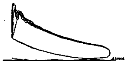
Fig. 137.—Hornsby-Akroyd Engine— Indicator Diagram.
