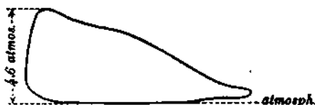
Fig. 18.—Simon Engine—Indicator Diagram.
