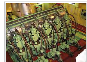
The MAN B&W 5S50MC 5-cylinder, 2-stroke, low-speed marine diesel engine. This particular engine is found aboard a 29,000 tonne chemical carrier.
