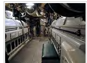
Fairbanks-Morse opposed piston diesel engines on the WWII submarine USS Pampanito (SS-383) (on display in San Francisco)
