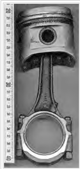
Piston, piston ring, gudgeon pin and connecting rod
