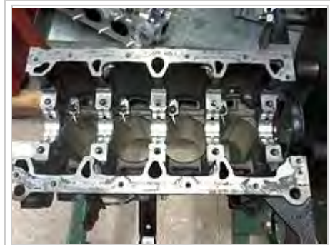
Engine block seen from below. The cylinders, oil spray nozzle and half of the main bearings are clearly visible.
