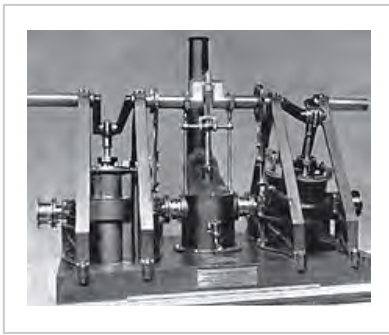
Model of a Maudslay oscillating engine
