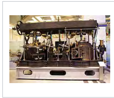
Oscillating engine built in 1853 by J. & A. Blyth of London for the Austrian paddle steamer Orsova
