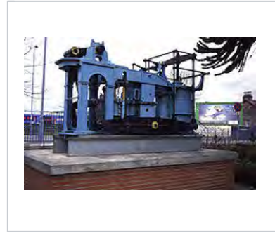
Early Napier side-lever engine from PS Leven , on display at Dumbarton, Scotland
