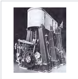
140-ton – also described as 135-ton – vertical triple-expansion engine of the type used to power World War II Liberty ships, assembled for testing prior to delivery. The engine is 21 feet (6.4 meters) long and 19 feet (5.8 meters) tall and was designed to operate at 76 rpm and propel a Liberty ship at about 11 knots (12.7 mph; 20.4 km/h).
