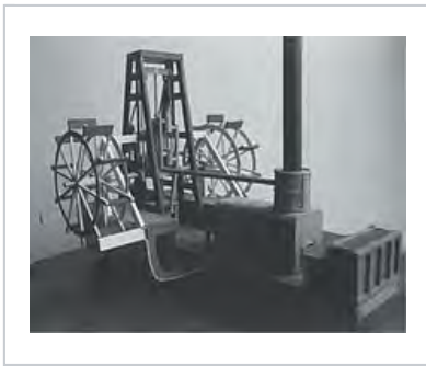
Model of a crosshead or "square" engine, showing location of engine cylinder above the crankshaft; also piston rod, crosshead, connecting rods and paddlewheels
