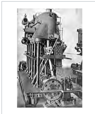
Vertical triple-expansion engine of USS Wisconsin (BB-9). The typical vertical engine arrangement of cylinder, piston rod, connecting rod and crankshaft can clearly be seen in this photo.
