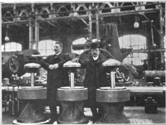
FIG. XIII. 65. Three Exhaust Valves for 2,000 H.P. Nürnberg Engine.
