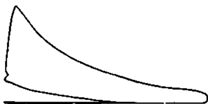
FIG. XIV.—10. Indicator Diagram showing faulty Cord Adjustment.
