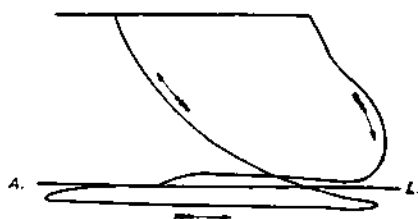
FIG. XV.—11. Resistance Diagram showing Scavenging by Fluid Inertia.
