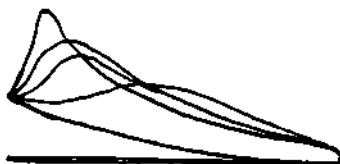
FIG. XI.—9. Indicator diagram showing loss of efficiency due to weak mixture.
