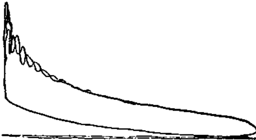
FIG. XIV.—20. Indicator Diagram showing Inertia Effect of Indicator Mechanism.
