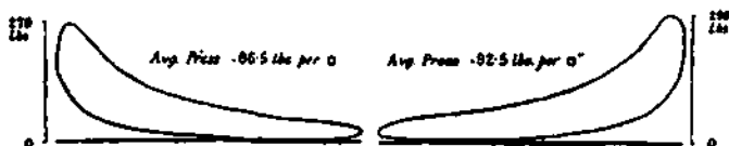
FIG. XV.—35. Diagrams from opposite ends of Cylinder of 1,000 H.P. Nürnberg Engine.
