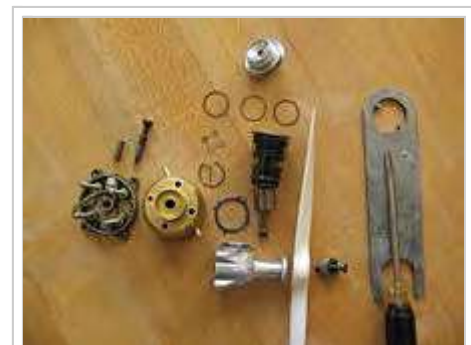
A Cox Babe Bee 0.049 cubic inch (0.8 cubic cm) reed valve engine, disassembled, uses glow plug ignition. The mass is 64 grams.
