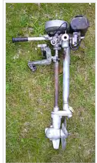
Lateral view of a two-stroke Forty series British Seagull outboard engine, the serial number dates it to 1954/1955
