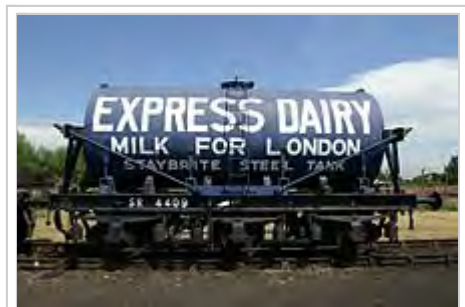
Preserved Express Dairies three-axle Milk Tank Wagon at the Didcot Railway Centre, based on an SR chassis
