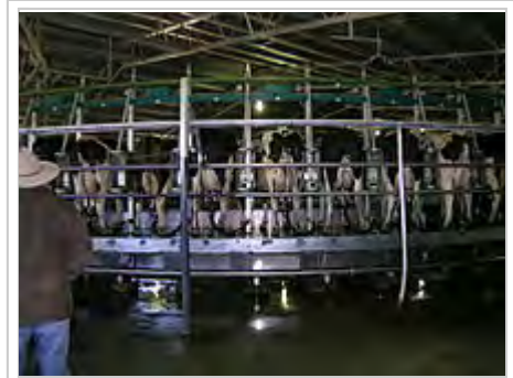
80-stand rotary dairy that is fully computerised and records milk production
