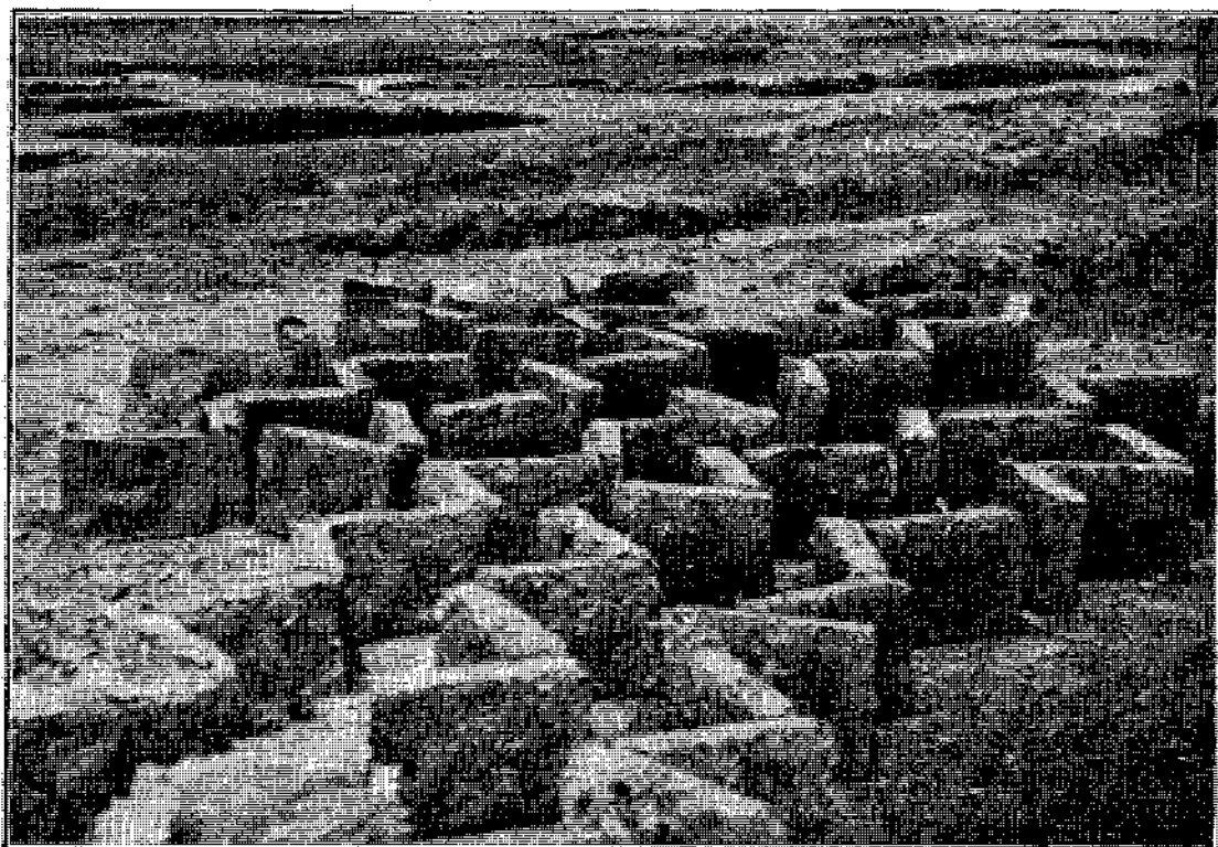
Fig. 89.—Air-dried earth brick for house building.
