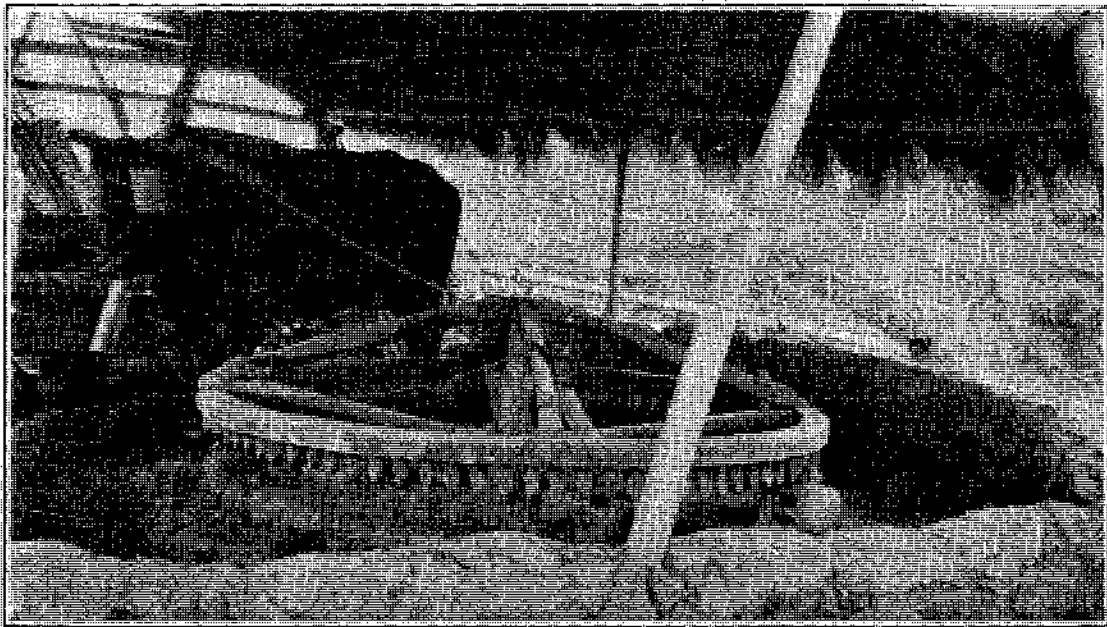
Fig. 158.—Close view of power wheel with cow attached, used in driving the irrigation pump, one of the two seen in Fig. 157.
