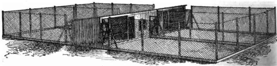
FIG. 205. Double poultry house and sheds: The sheds are shown at the ends, the roosting rooms in the center. This plan permits of any number of such houses, the interior arrangement being shown in Figs. 206 and 207. (Plan submitted by Mr. M. K. Boyer, Hammonton, N. J.)
