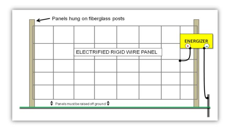
Figure 5. Electrified raised rigid wire panel
