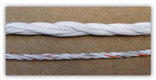
Figure 4. Two styles of electrical fencing "Poly" wires.
