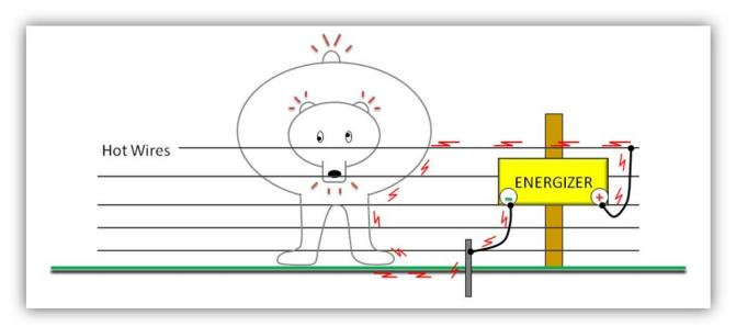
Figure 1. A bear completes the electrical circuit and receives a shock
