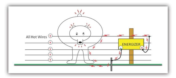
Figure 2. An all-hot electric fence design. All wires are connected to each other and to the positive terminal on the energizer.
