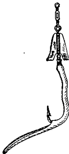
Fig. 47. Rubber Eel complete, with spinner and swivel. Loop of gut collar is attached to the upper eye of swivel.
