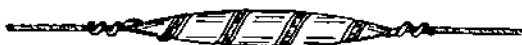
Fig. 28. "Archer-Jardine" Lead, placed upon the line by colling it round the grooves.
