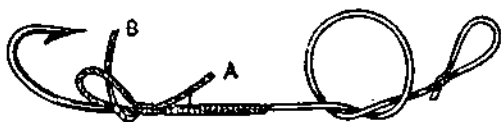
Fig. 36. Finishing Off the Whipping, accomplished by forming a loop with A, passing three coils over it with B, and inserting the latter end. By drawing at A the loop is pulled beneath the whipping.
