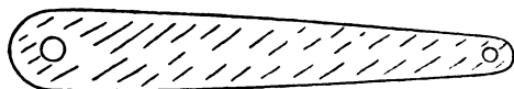
Fig. 70. Boom for Plummeting enlarged, the larger hole being intended to receive the main line, and the smaller for attaching the snooding.
