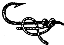
Fig. 8. Attaching Fine Snooding to a Hook, two half-hitches being passed over the shank and a third over the bend.
