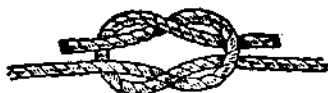
Fig. 105. Reef Knot, with turns slack. To commence, the right end should be placed under the left.
