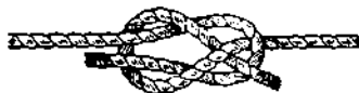
Fig. 106. Sheet Bend, formed by making a loop in one rope. The other end is then introduced, brought round the back of the loop, and placed under its own part.
