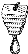
Fig. 118. Cork-Buoy, with knotted rope at top and bottom, and large spliced loop below.
