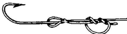
Fig. 34. Double Slip-Knot attachment for Gut, formed by putting the end through the eye twice as here shown, and then by tying one-half of a double Fisherman's Knot upon main part.
