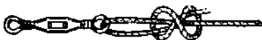
Fig. 66. Attaching Snooding to the eye of a Swivel, performed by passing the end through the eye, taking two turns over the left fore-finger, and putting the end backwards through the coils.
