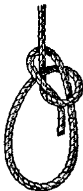
Fig. 107. Bowline, a most useful method of forming a bight at the end of a rope.
