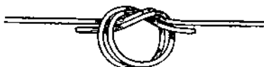
Fig. 5. The Single Overhand Knot with two parts for Gut Collar, made by tying a single knot over both strands.
