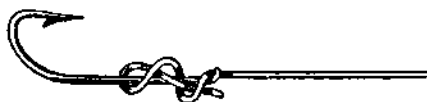
Fig. 32. Double Jam Knot for connecting Gut, the end being brought twice round the shank and then introduced beneath both coils.
