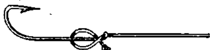
Fig. 31. Simple Jam Knot for attaching Gut to eyed hook, a knot being tied at the extremity to prevent slipping after passing the end through the eye.
