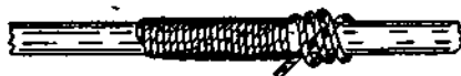
Fig. 22. Method of Finishing Whipping, dotted lines showing the direction of the joint.
