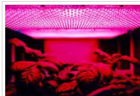
Red LED lights illuminate potato plants in a NASA study on growing food in space
