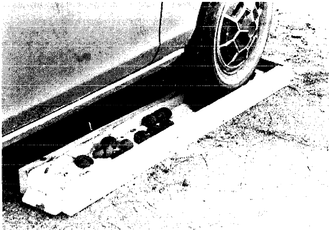
This wooden trough, built especially for the purpose, allows you to use your car to hull black walnuts. Without the trough the nuts shoot out from under the car's tire, without cracking.
