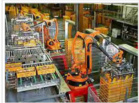
Automated palletizer of bread with industrial KUKA robots at a bakery in Germany
