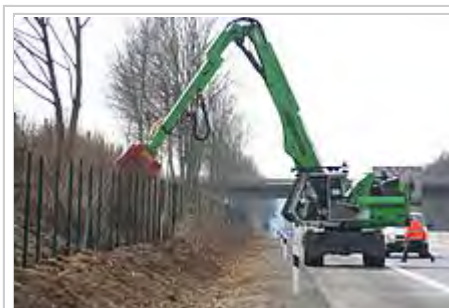
Fecon mulching attachment on a Sennebogen excavator, being used to clear roadside brush in Germany
