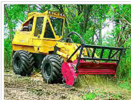
Hydraulic-powered mulching attachment on rubber-tired tractor
