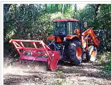
PTO-driven forestry mulching attachment on an agricultural tractor
