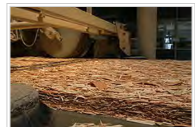
Production of oriented strand board.
