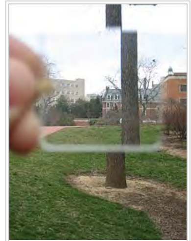
A wedge prism showing a borderline tree.
