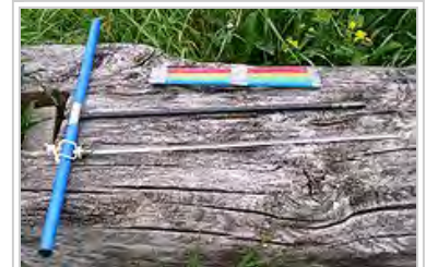
An increment borer with common drinking straws, a cost-effective manner often used to hold derived cores.
