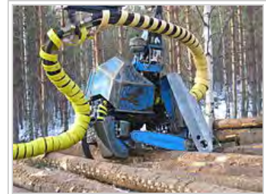
The boom of a cut-to-length harvester with attached chainsaw cutting Pinus sylvestris in Finland.
