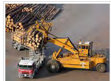
A loader lifting logs off a semi at Port Chalmers, within the city of Dunedin, New Zealand.
