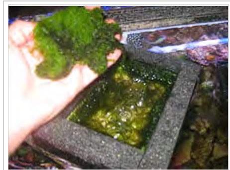
Seaweed is lifted out of top of algae scrubber/cultivator, to be discarded or used as food, fertilizer, or skin care
