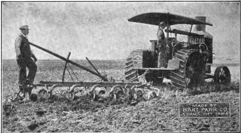
FIG. 112. — HART-PARR GASOLINE TRACTION ENGINE.
