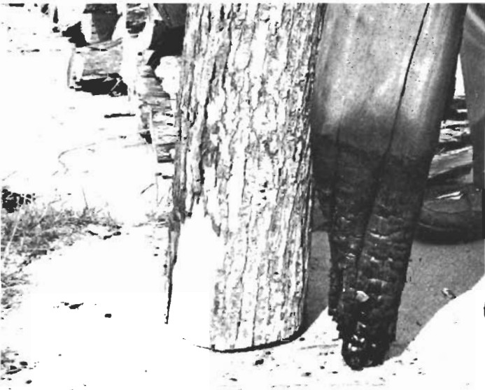
Wood burns in the refractory zone only.
