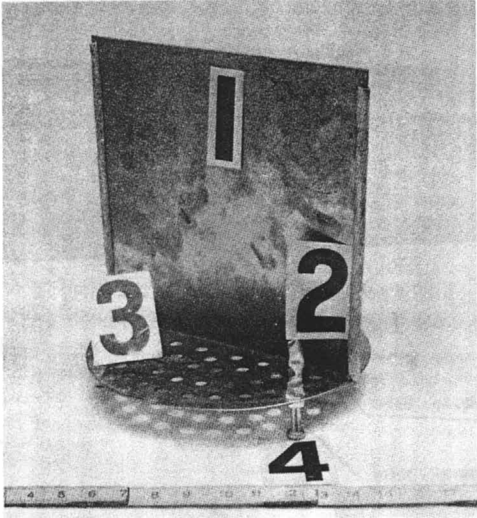
Fig. 2-17. Divider plate (#1) and bottom plate (#3), with standoffs (#4), for the filter unit. Note the high-temperature hose lining the sides of the divider plate.
