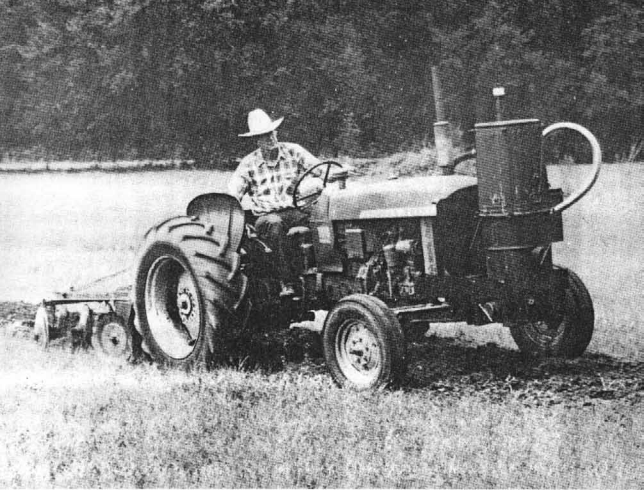
Fig. S-3. Wood gas generator unit in operation during field testing.
