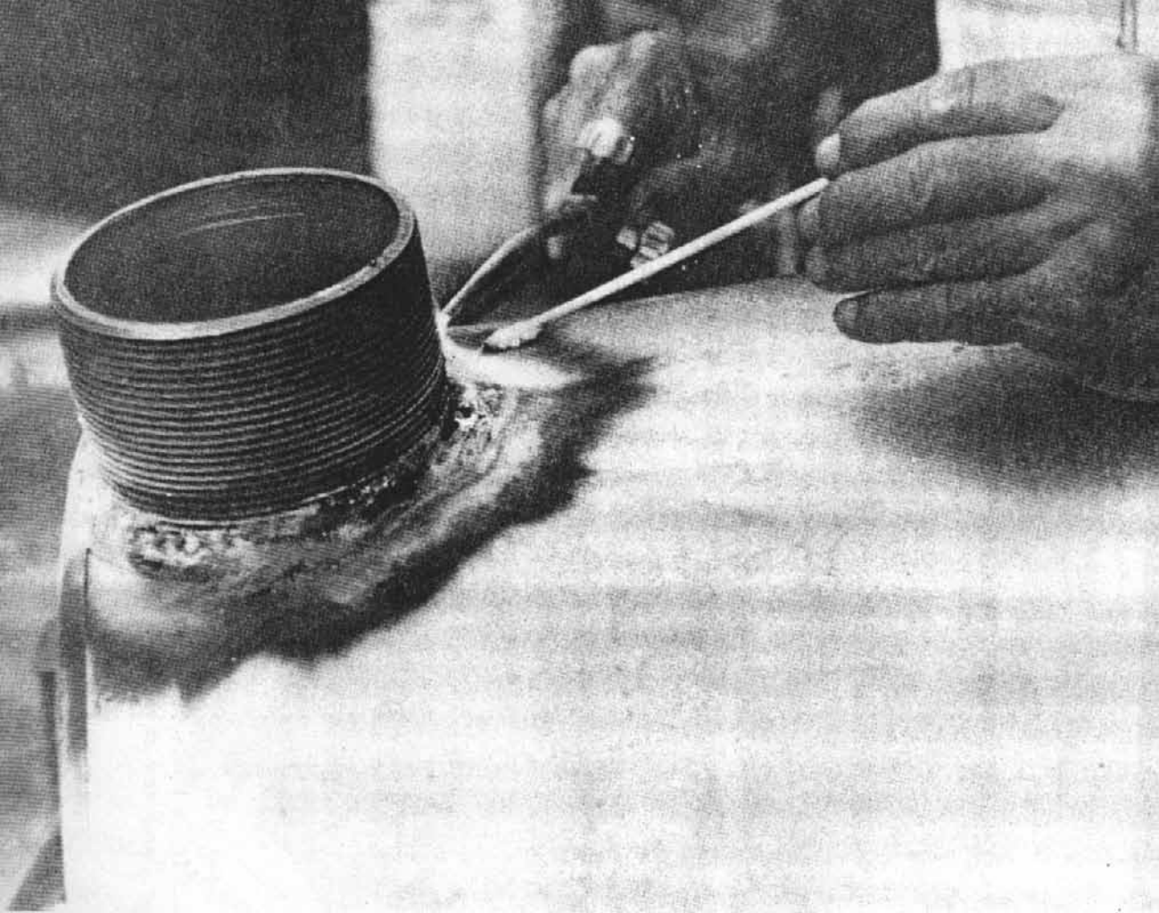
Fig. 2-7. Braze, do not weld , the plumbing fittings to the thin walled drums.
