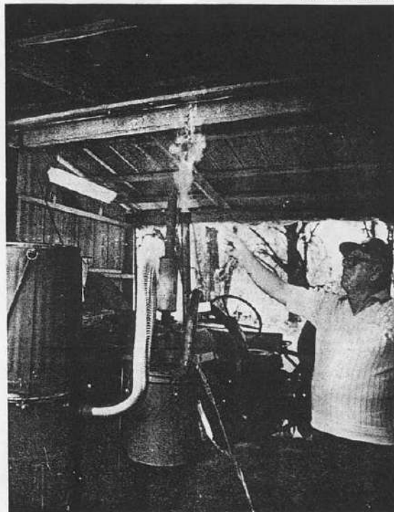
Fig. 3-3. Igniting the exhaust gas will demonstrate that the gasifier unit is working properly.
